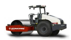
CA300 is a typical utility machine, designed for long working days in tough applications. It is utilized for compaction of most types of soil. Typical applications are road building, airfields, dams, harbors and industrial sites. The CA300 is available with smooth drum as well as padfot drum with or without drum drive.
