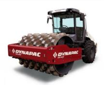
CA250 is a typical utility machine, designed for long working days in tough applications. It is utilized for compaction of most types of soil. Typical applications are road building, airfields, dams, harbors and industrial sites. The CA250 is available with smooth drum as well as padfot drum with or without drum drive.
